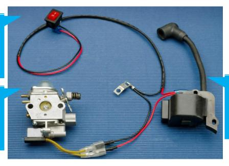
Walbro digital ignition system automatically adjusts spark timing and fuel delivery based on engine
