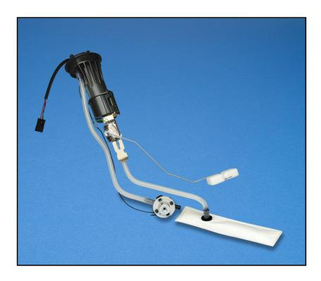
Walbro Fuel Pump Assemblies are designed to fit the needs of our customer's various fuel tank configurations while meeting the required fuel flow, pressure, and packaging requirements.
