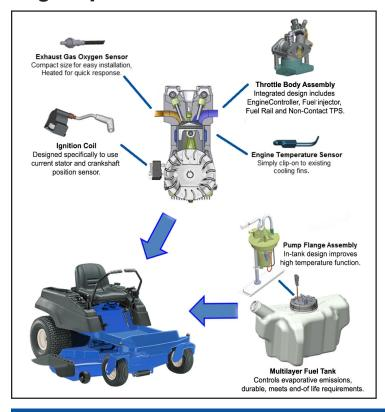
Walbro's EEM™ Injection System replaces the carburetor with an affordable Electronic Fuel Injection system developed specifically for small engines.
