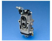
The WYA is a metal-bodied, rotary valve carburetor designed for stratified scavenging engines with 20 to 50 cc displacement. Meets all CARB and EPA regulations.
