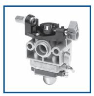
The WYB is a metal bodied rotary valve carburetor designed for 2 stroke engines less than 25 cc and 4 stroke engines less than 30 cc. This model is specifically designed for hand held 4 stroke engines featured on many power tools. Meets all C.A.R.B. and EPA emissions regulations.
