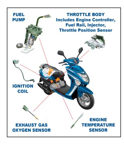
Walbro's EEM<sup>™</sup> Injection System replaces the carburetor with an affordable electronic fuel injection system.
